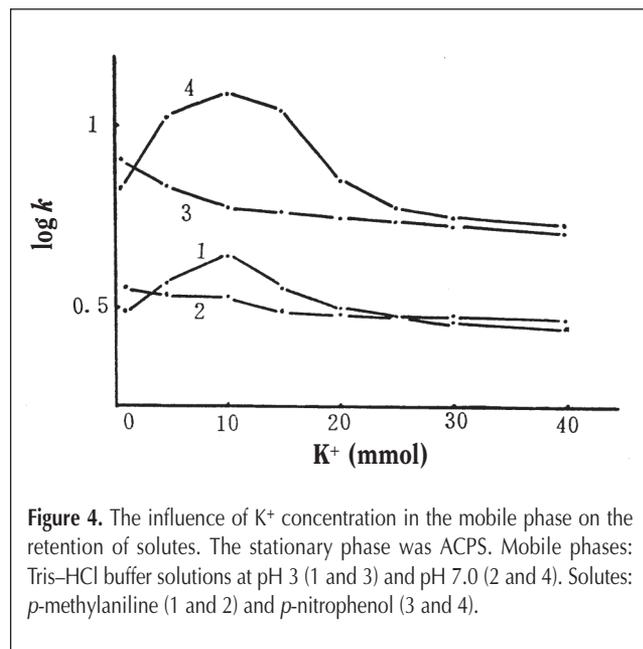
**Figure 4.** The influence of  $K^+$  concentration in the mobile phase on the retention of solutes. The stationary phase was ACPS. Mobile phases: Tris-HCl buffer solutions at pH 3 (1 and 3) and pH 7.0 (2 and 4). Solutes: *p*-methylaniline (1 and 2) and *p*-nitrophenol (3 and 4).
