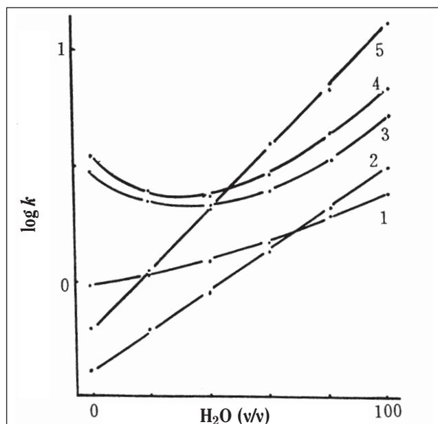
**Figure 2.** Plot of logarithms of capacity factors on the bonded phases versus the content of methanol in the mobile phase. The solute was *p*-nitrophenol. Stationary phases: 1, DEAP; 2, CPS; 3, ACPS(I); 4, ACPS(II); 5, ODS.
