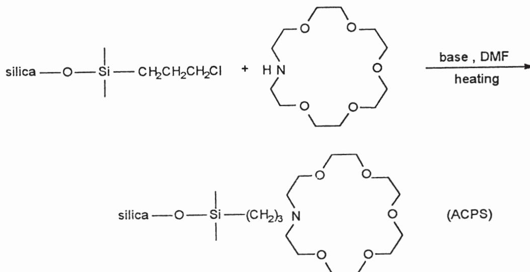
Figure 1. Reaction sequence used to prepare the bonded phases.
