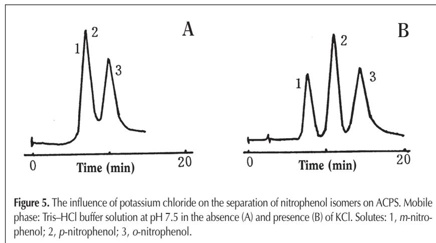
**Figure 5.** The influence of potassium chloride on the separation of nitrophenol isomers on ACPS. Mobile phase: Tris-HCl buffer solution at pH 7.5 in the absence (A) and presence (B) of KCl. Solutes: 1, *m*-nitrophenol; 2, *p*-nitrophenol; 3, *o*-nitrophenol.
