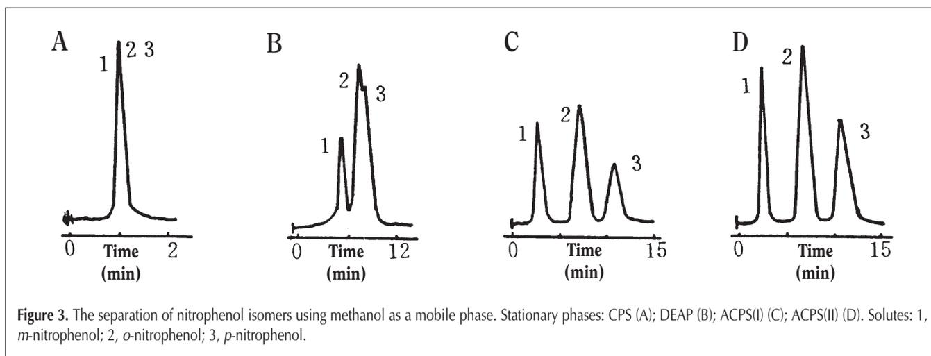
Figure 3. The separation of nitrophenol isomers using methanol as a mobile phase. Stationary phases: CPS (A); DEAP (B); ACPS(I) (C); ACPS(II) (D). Solutes: 1, *m*-nitrophenol; 2, *o*-nitrophenol; 3, *p*-nitrophenol.
